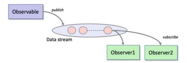
In the above figure, the Observable object publishes data to a Data Stream. The data in the Data Stream is then sent to each of the Observers registered with the Observable. In this way data is broadcast to all Observers of an Observable.
