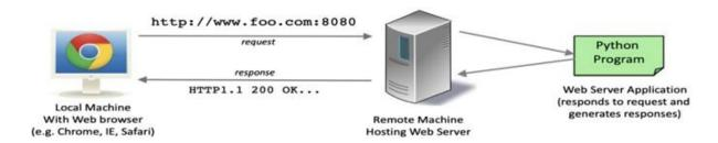
In the above diagram the user is using a browser (such as Chrome, IE or Safari) to access a web server. The browser is running on their local machine (which could be a PC, a Mac, a Linux box, an iPad, a Smart Phone etc.).
