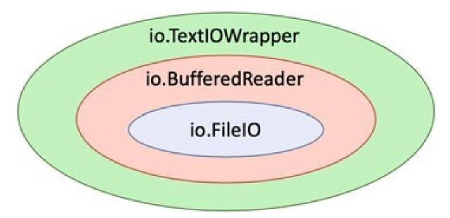
In the above figure the initial FileIO stream reads raw data from the actual data source (in this case a file). The BufferedReader then buffers the data reading process for efficiency. Finally the TextIOW rapper handles string encoding; that is it converts strings from the typical ASCII representation used in a file into the internal representation used by Python (which uses Unicode).
