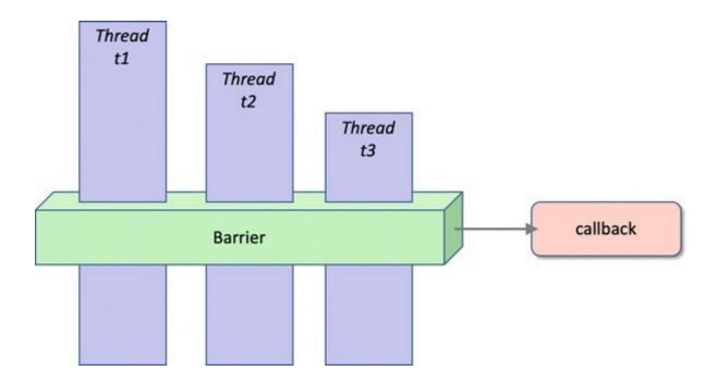
An example of using a Barrier object is given below. Note that the function being invoked in each Thread must also cooperate in using the barrier as the code will run up to the barrier.wait() method and then wait until all other threads have also reached this point before being allowed to continue.
