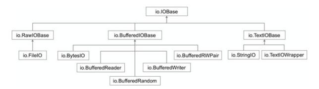
The abstract IOBase class is at the root of the stream IO class hierarchy. Below this class are stream classes for unbuffered and buffered IO and for text oriented IO.
