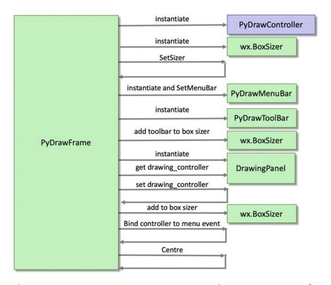
ThePyDrawFrame constructor sets up the environment for the application. It creates the top level PyDrawController. It creates the DrawingPanel and initializes the display layout. It initializes the menu bar and tool bar. It binds the controllers menu handler to the menus and centers itself.
