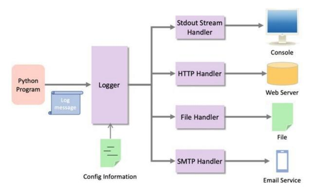
In the above diagram the logger has been configured to send all log messages to four different handlers which allow a log message to be written to the console, to a web server to a file and to an email service. Such a behavior may be required because:
