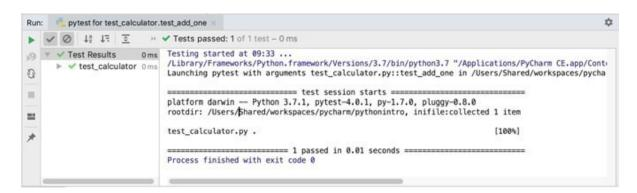
Here you can see a tree in the left-hand panel that currently holds the one test defined in the test\_calculator.py file. This tree shows whether tests have passed or failed. In this case we have a green tick showing that the test passed.
