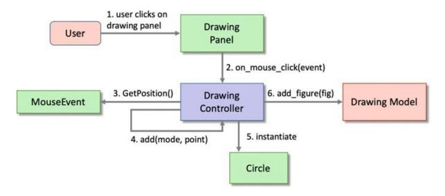
The above illustrates what happens when the user presses and releases a mouse button over the drawing panel, to create a new figure. When the user presses the mouse button, a mouse clicked message is sent to the DrawingController, which decides what action to perform in response (see above). In PyDraw, it obtains the cursor point at which the event was generated by calling the GetPosition() method on the mouse\_event.
