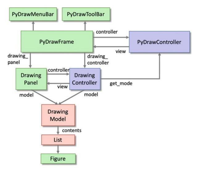
The PyDrawFrame is responsible for setting up the controller and the DrawingPanel. The PyDrawController is responsible for handling menu and tool bar user interactions. This separates graphical elements from the behavior triggered by the user.
