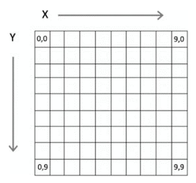
The above diagram illustrates how pixels within a Surface are indexed. Indeed a Surface can be used to draw lines, shapes (such as rectangles, squares, circles and ellipses), display images, manipulate individual pixels etc. Lines are drawn from one pixel location to another (for example from location 0,0 to location 9,0 which would draw a line across the top of the above display surface). Images can be displayed within the display surface given a starting point such as 1, 1.
