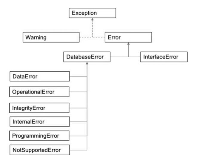
The above diagram illustrates the inheritance hierarchy for the errors and warning associated with the standard. Note that the DB-API Warning and Error both extend the Exception class from standard Python; however, depending on the specific implementation there may be one or more additional classes in the hierarchy between these classes. For example, in the PyMySQL module there is a MySQLError class that extends Exception and is then extended by both
