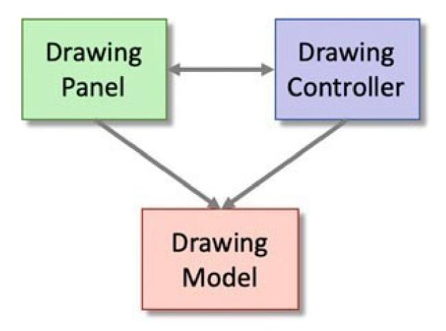
The DrawingModel, DrawingPanel and DrawingController classes exhibit the classic MVC structure. The view and the controller classes (DrawingPanel and DrawingController) know about each other and the drawing model, whereas the DrawingModel knows nothing about the view or the controller. The view is notified of changes in the drawing through the paint event.
