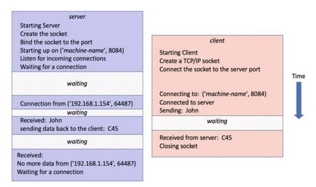
As you can see from this diagram, the server waits for a connection from the client. When the client connects to the server; the server waits to receive data from the client. At this point the client must wait for data to be sent to it from the server. The server then sets up the response data and sends it back to the client. The client receives this and prints it out and closes the connection. In the mean time, the server has been waiting to see if there is any more data from the client; as the
