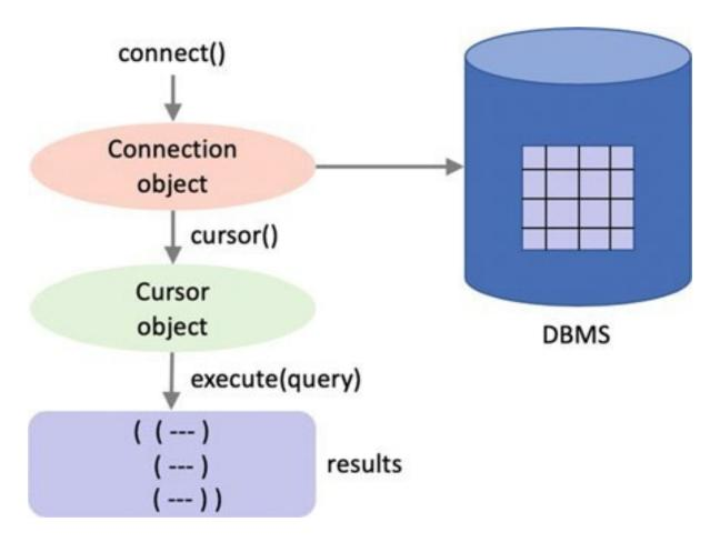
The standard specifies a set of functions and objects to be used to connect to a database. These include the connection function, the Connection Object and the Cursor object.
