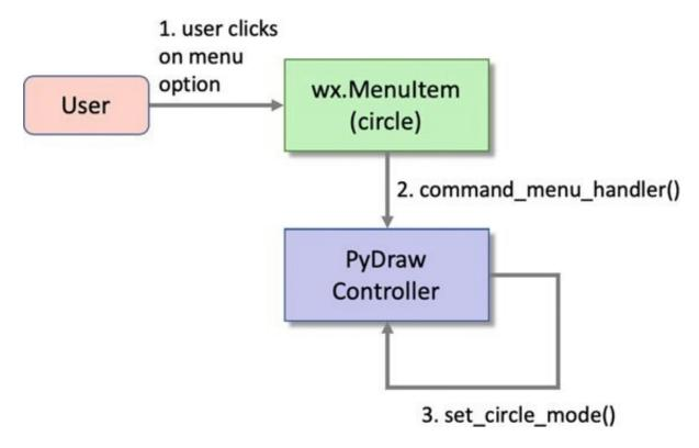
When the user selects one of the menu items the command\_menu\_handler of () method the PyDrawController is invoked. This method determines which menu item has been selected; it then calls an appropriate method (such set circle mode() setter as or set\_line\_mode() etc.). These methods set the mode attribute of the controller to an appropriate value.
