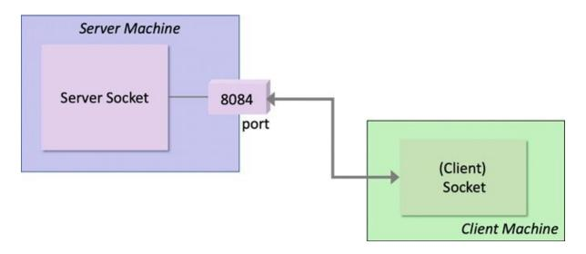
For example, in the above diagram the server socket connects to port 8084. In turn the client socket connects to the machine on which the server is executing and to port number 8084 on that machine.
