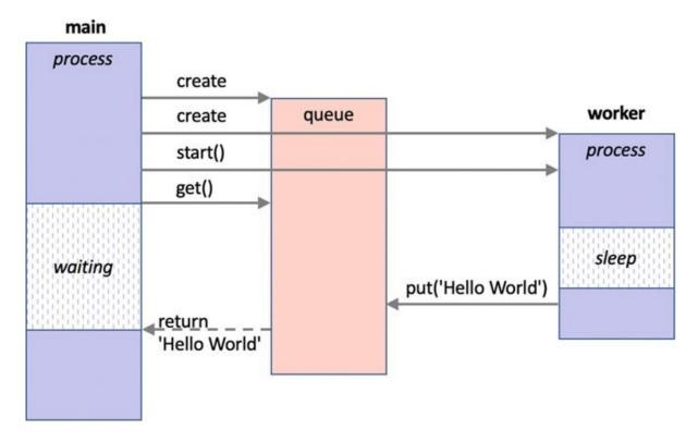
In the above diagram the main process waits for a result to be returned from the queue following the call to the get() method; as it is waiting it is not using any system resources. In turn the worker process sleeps for two seconds before putting some data onto the queue (via put('Hello World')). After this value is sent to the Queue the value is returned to the main process which is woken up (moved out of the waiting state) and can continue to process the rest of the main function.
