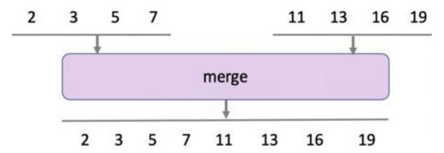
In the above diagram two Observables are represented by the sequence 2, 3, 5, 7 and the sequence 11, 13, 16, 19. These Observables are supplied to the merge operator that generates a single Observable that will supply data generated from both of the original Observables. This is an example of an operator that does not take a function but instead takes two Observables.
